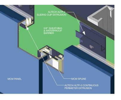
The Accu-Trac® DS System is a dry-joinery system utilizing standard ½" reveals to emphasize the vertical and horizontal joints in lieu of exposed sealants. The DS system provides ease of installation with our patented sliding clip technology. Custom reveals with variable dimensions are also available. A nearly endless variety of colors, natural metals, wood grains and faux stone finishes are available which allows this system to be utilized in a multitude of applications to fit any design!
