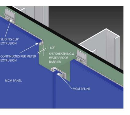
The **Low Profile DS** system is a 1-1/2" deep, back ventilated rainscreen system with an integral spline. This system is not only designed as a cost saving alternative to conventional systems, but its low-profile allows it to be used in areas where system depth is limited. A nearly endless variety of colors, wood grains, faux stone and natural metal finishes means the Low Profile DS system can be used for either interior or exterior applications and fit **any** design!
