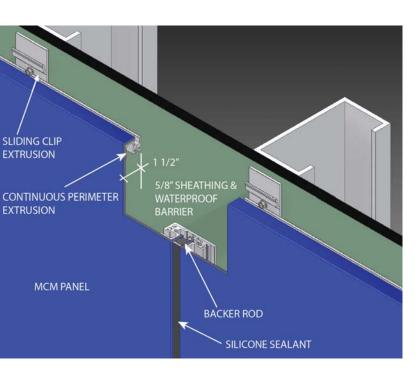
The **Low Profile ES** system is a 1-1/2" deep, exposed sealant system. This system is not only designed as a cost saving alternative to conventional systems, its low-profile allows it to be used in areas where system depth is limited. A nearly endless variety of colors, wood grains, faux stone and natural metal finishes means our Low Profile ES system can be used for either interior or exterior applications to fit **any** design!
